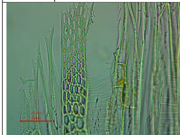
Tangent 40X: note intercellular spaces between ray cells and helical thickenings. Intercellular spaces are not necessarily diagnostic but noted for future research
