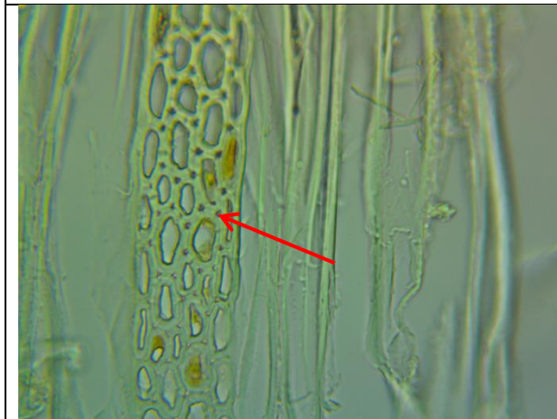
Tangent 60X: note intercellular spaces between ray cells. Not necessarily diagnostic but noted for future research
